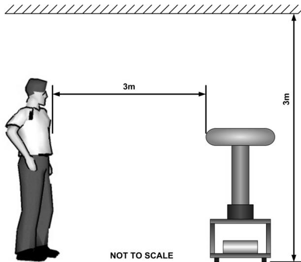
**Figure 2. Required clearances for operation**
