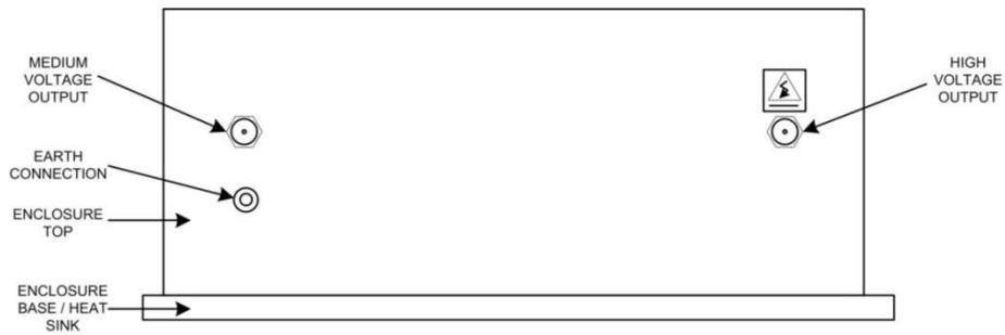
**Figure 6. Rear of power supply**
