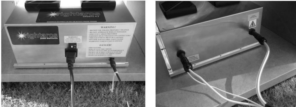
**Figure 7. Wiring connections of the power supply**
