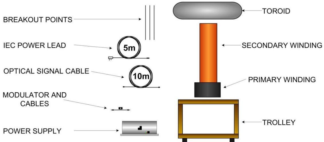
**Figure 1. Coil components**
